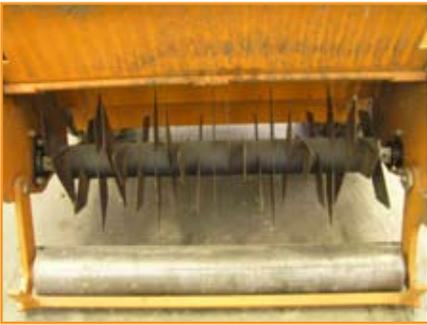
cutting blades from 3/64 to 3/8 inch thick are spaced vertically (e.g., 1 inch on center) on a shaft horizontal to the soil surface. Rows of exposed soil form as these machines move across the turf. Larger, tractor-drawn linear aerators are also available. Linear aeration may expose much more of the soil surface area than core aerification.
