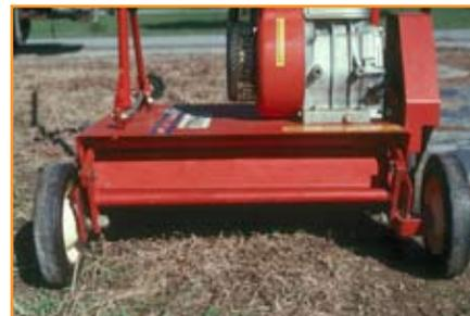
spinning, horizontal shaft may be used to relieve 'grain,' dethatch or cultivate turf. For example, grain is reduced when the knives are set to sever aboveground runners
